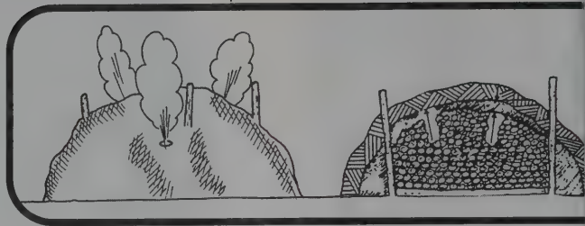
Charcoal-making oven. Cross-section of stacked virgin wood with air tubes; covered by mud to seal out air and burn slowly.
